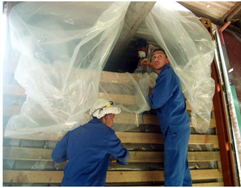
Open faced liner – loading fish meal via a screw feeder
